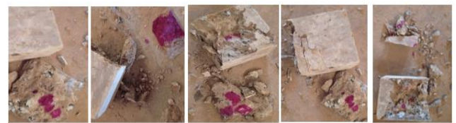
Fig. 11. Carbonation resistance results of normal and SA concrete mixtures
