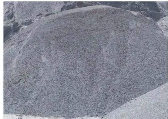
Crushed stone dust (sand) as fine aggregate
