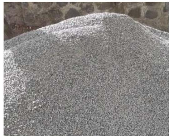
Crushed granite as coarse aggregate
