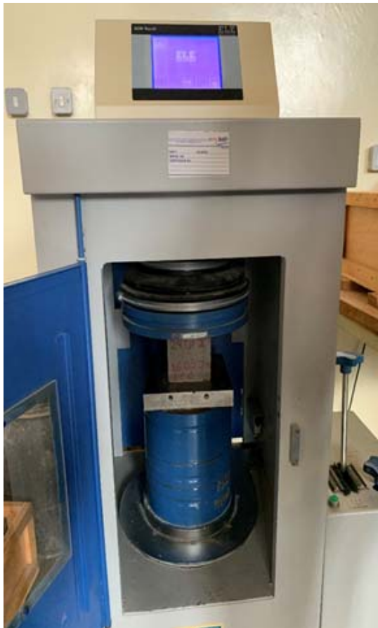
Fig. 2: Test setup of concrete cubes for compressive strengths.
