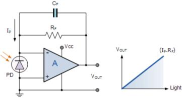
A photo-current-to-voltage converter circuit uses an operational amplifier as an amplifying device. The output voltage  $V_{out} = I_P * R_f$  is proportional to the light intensity. It can turn its current flow both "ON" and "OFF" in nanoseconds.
