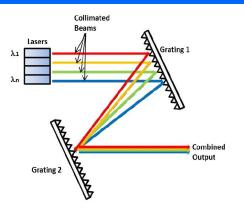
The external resonant cavity is formed by an output coupler that returns a fraction of the power back to each laser with a second reflection from the grating. The design is shown in above figure.
