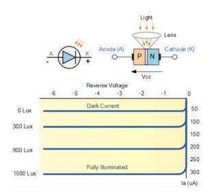
When used as a light sensor, a photodiodes dark current (0 lux) is about 1uA for silicon type diodes. When light falls upon the junction more hole/electron pairs are formed and the leakage current increases.
