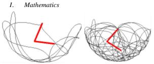
A set of calculus equations in physics relating to double pendulums govern the Swinging Sticks. According to the Runge-Kutta methods of numerical analysis, it is regarded as a compound double pendulum that swings in a 2D plane.
