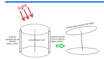
*E.* How the pendulum motion can keep tracking with the flying object?
