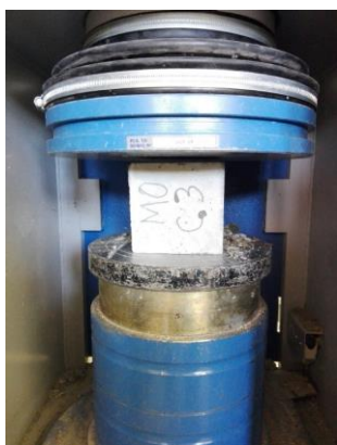
Fig. 4: Compressive strength test
