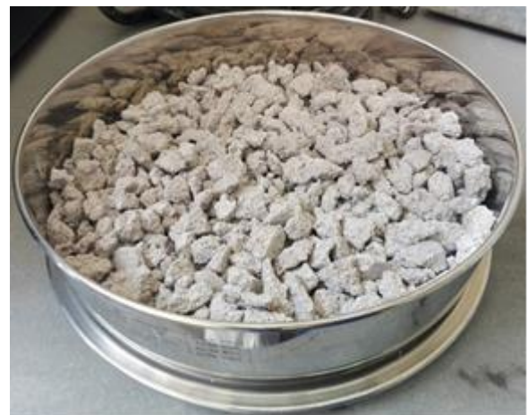
Fig. 3: Graded recycled coarse aggregate
