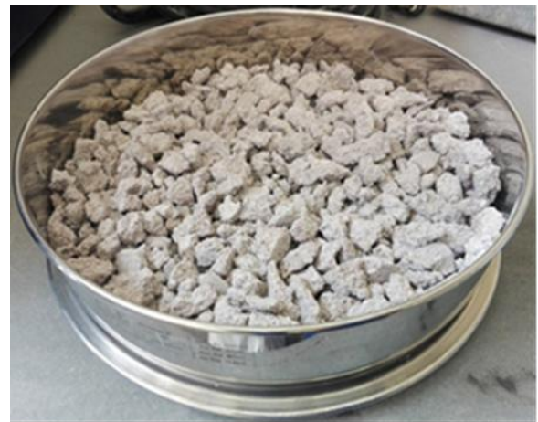
Fig. 3: Graded recycled coarse aggregate
