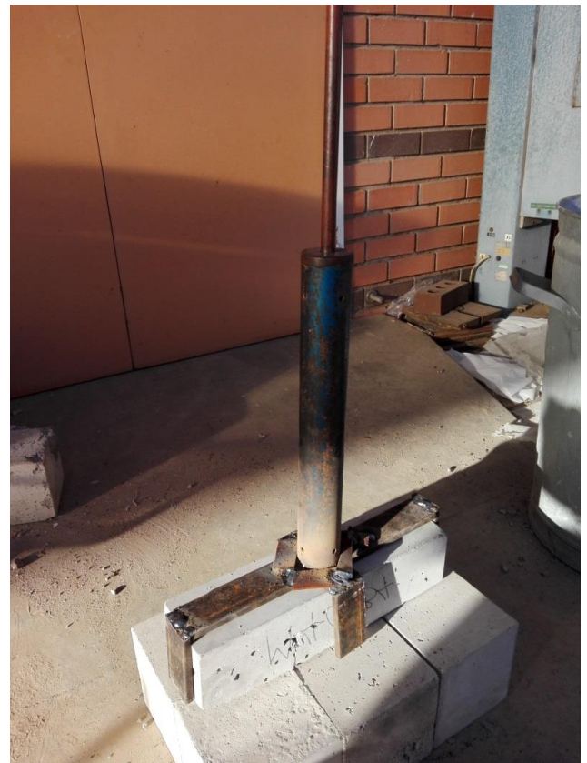
Fig. 4: Free falling weight test and concrete beam
