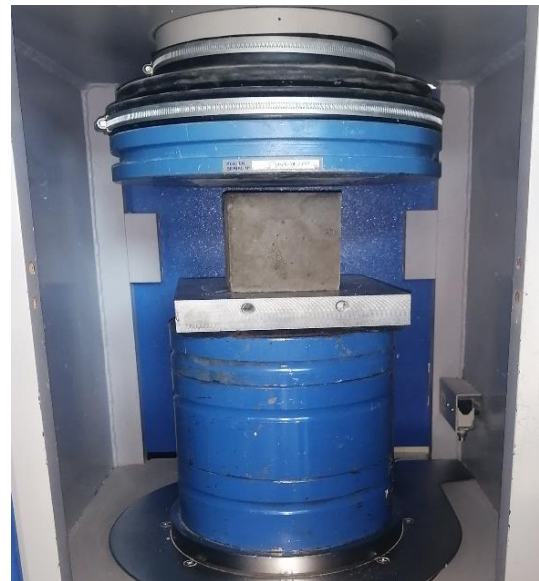
Fig. 4: Test setup of concrete cubes for compressive strengths.
