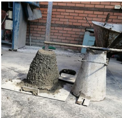
Fig. 3: Slump test set-up
