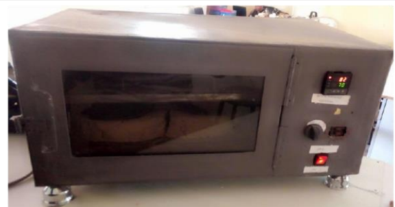
Fig. 4: The Portable Cocoa bean dryer cabinet design and outlook
