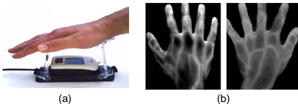
FIG.2: HAND VEINS(A) DEVICE USED, (B) INFRARED IMAGES OF THE BACK OF TWO DIFFERENT HANDS TAKEN IN A NORMAL OFFICE ENVIRONMENT
