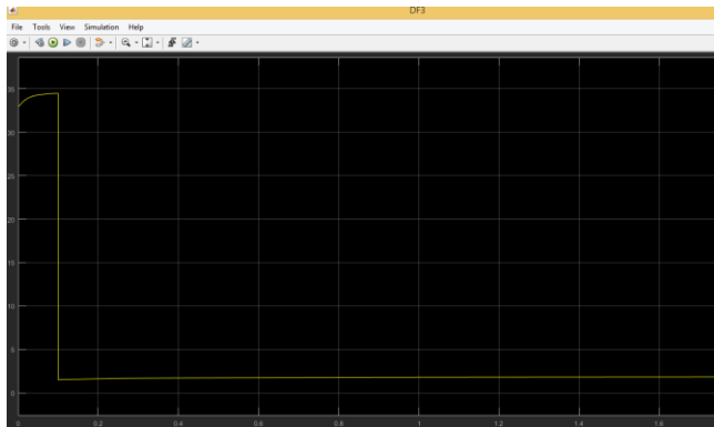
Fig. 9. Robot Angle Response to Disturbance Force
