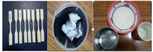
Fig 4: (a) SLA Printed specimen (b) Specimen wrapped in black paper (c) Specimen during curing.
