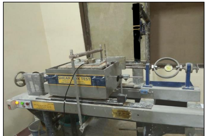
Fig. 1: Large-scale direct shear box test apparatus
