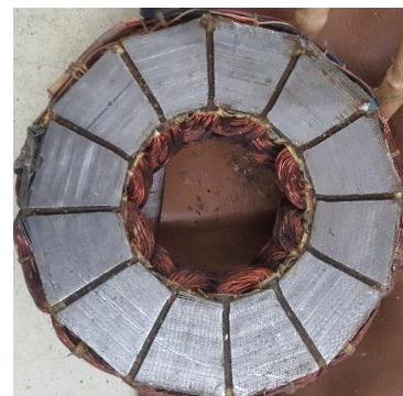
Figure 1 Stator consist of core and armature
