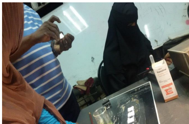
Plate 3. ZnO thin-film (electrode) dipped into the Coumarin 500 and Yamidine dyes.
