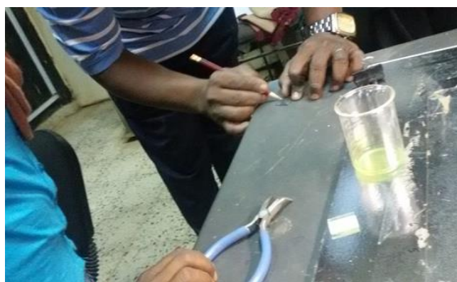
Plate 2. Conducting surface of ITO slide coated with graphite of a dark pencil.
