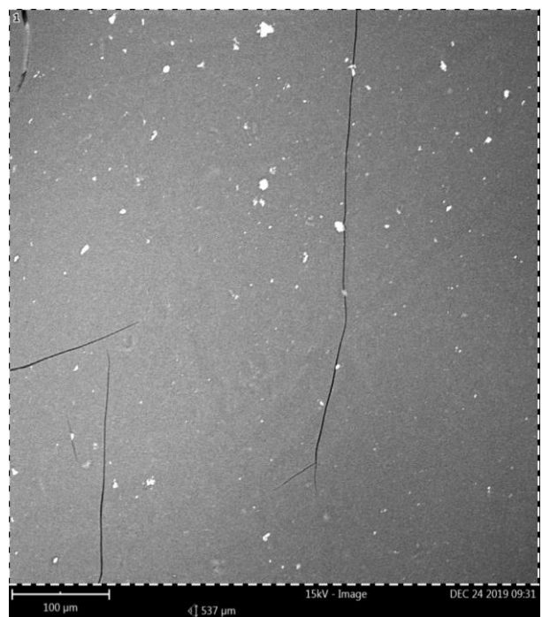
Figure 3.4(b): Scanning Electron Microscopy of Ipomea batatas adhesive in the presence of PVAc.
