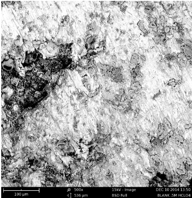
Fig.3.0.(c) Micrograph for MS in 0.5M HClO 4 without CTE
