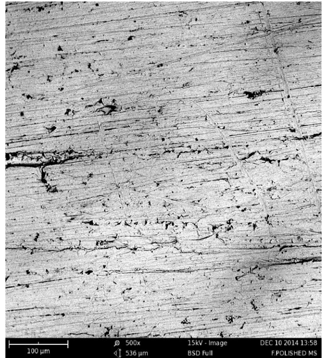
Fig. 3.0.(a) Micrograph for Freshly Polished MS before immersion
