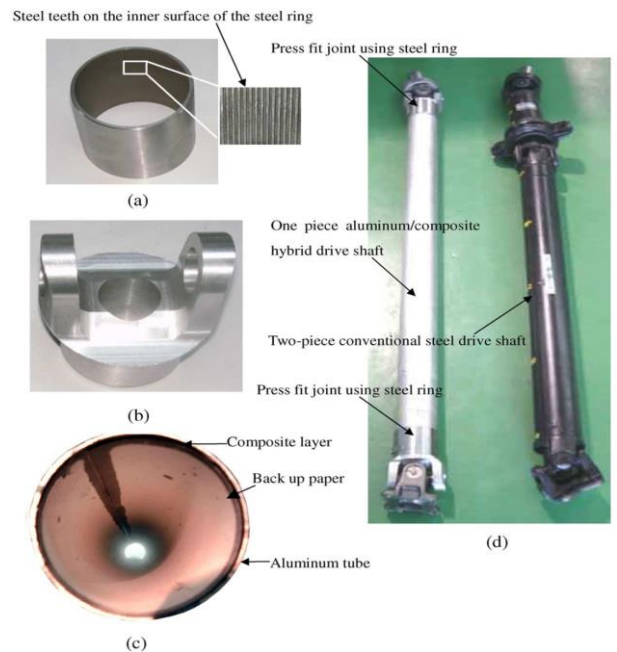
Fig 3: (a) Steel ring with inner surface having teeth in the axial direction; (b) aluminium yoke; (c) manufactured aluminium/composite hybrid tube; (d) manufactured one piece aluminium/composite drive shaft and conventional two-piece steel drive shaft.
