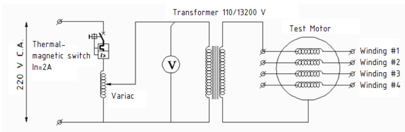
Fig. 1: Test circuit #1
