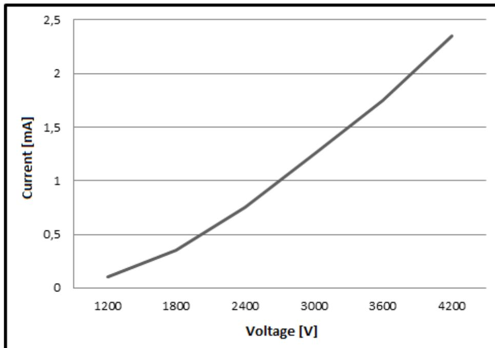
Fig. 5: Voltage vs current plot (L.V. side)
