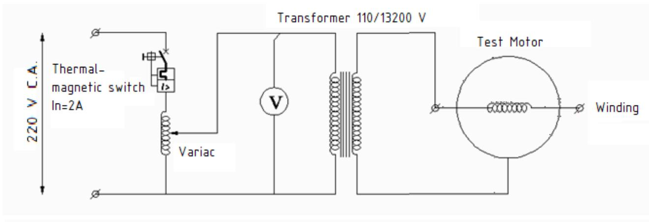
Fig. 2: Test circuit. Test #2
