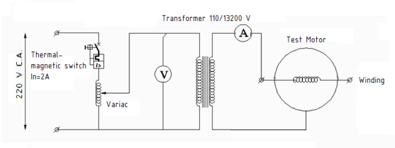
Fig.4: Test circuit. Measures on H.V. side
