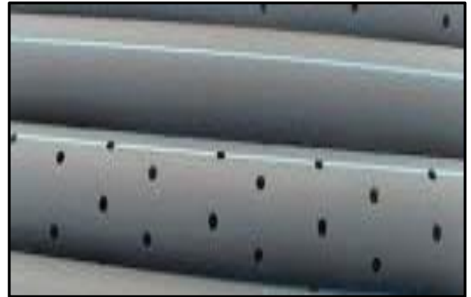
Figure 3: Sample of PVC pipe to measure water loss
