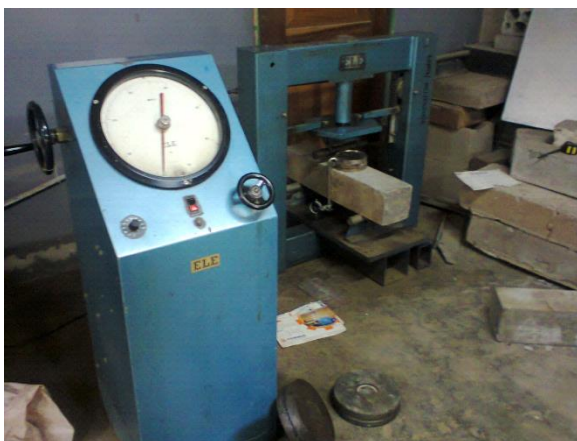
Fig. 3. Experimental setup of RC beam for flexural strength test.
