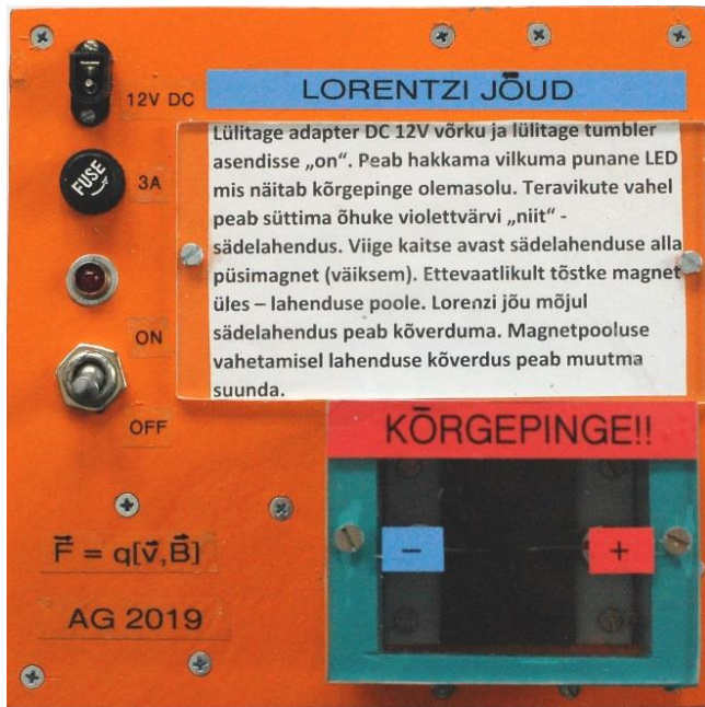
Fig.1. Appearance of the device for the demonstration of Lorentz force.
