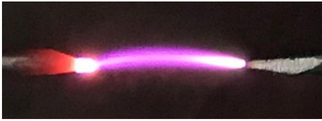
Fig.3. Shape of the spark discharge in the absence of a magnetic field.
