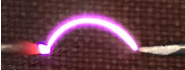
Fig.4. Shape of the spark discharge when a magnet is installed under it.
