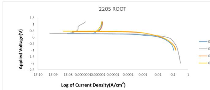
Figure 9: Potentiodynamic curves showing the corrosion behavior of Duplex stainless steel 2205 in  $H_2SO_4$  containing Nanoparticles from Root of *Solanum tuberosum* at different concentration.
