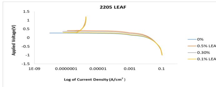
Figure 7: Potentiodynamic curves showing the corrosion behaviour of Duplex stainless steel 2205 in  $H_2SO_4$  containing Nanoparticles from leaf of *Solanum tuberosum* at different concentration.
