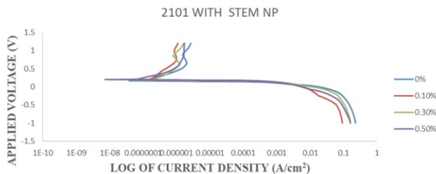
Figure 5: Potentiodynamic polarization curves for 2101 duplex stainless steel immersed in 0.5M H<sub>2</sub>SO<sub>4</sub> with and without potato stem extract as inhibitor.
