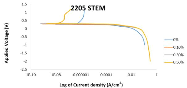
Figure 8: Potentiodynamic curves showing the corrosion behaviour of Duplex stainless steel 2205 in  $H_2SO_4$  containing Nanoparticles from Stem of *Solanum tuberosum* at different concentration.
