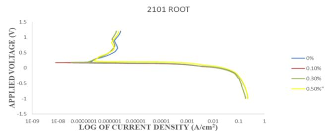
Figure 6: Potentiodynamic polarization curves for 2101 duplex stainless steel immersed in 0.5M H<sub>2</sub>SO<sub>4</sub> with and without potato root extract as inhibitor
