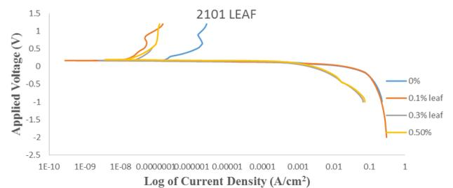
Figure 4: Potentiodynamic polarization curves for 2101 duplex stainless steel immersed in  $0.5\text{M H}_2\text{SO}_4$  with and without potato leaf extract as inhibitor.
