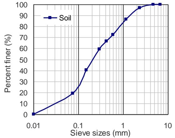
Fig. 2. Particle size distribution of soil sample ( $\leq 75 \mu m$ )
