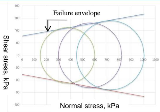
Fig. 6. Mohr circle diagram of soil samples under triaxial pressure
