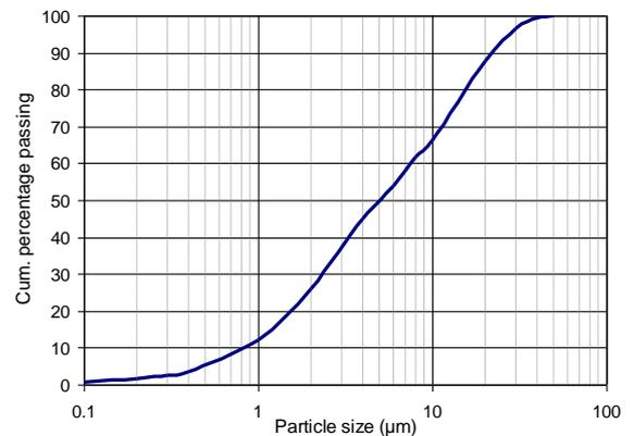
Fig. 3. Particle size distribution of soil ( $\leq 75 \mu m$ )
