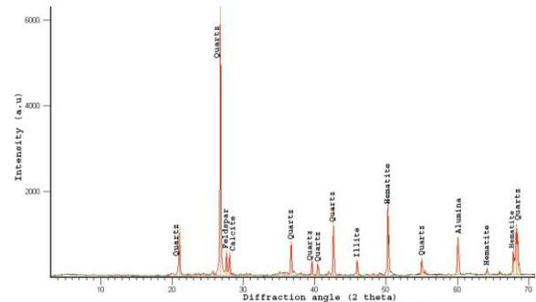
Fig. 1. XRD pattern of clay samples
