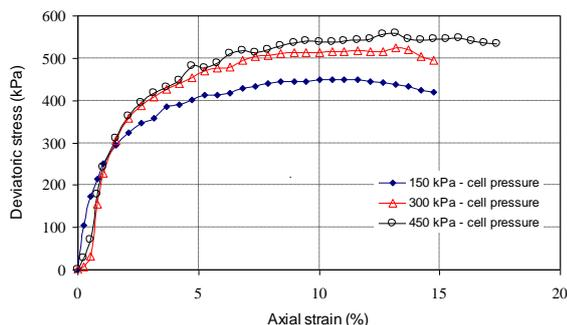
Fig. 7. Deviatoric stress-axial strain relation from triaxial testing of clay samples
