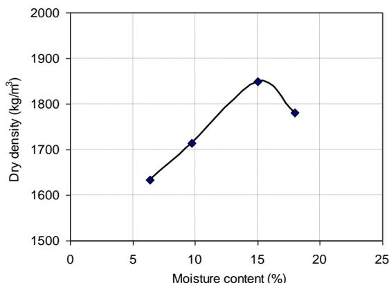
Fig. 4. Dry density vs moisture content curve from the compaction test results
