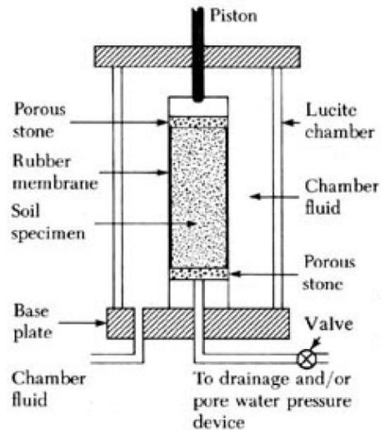
Fig. 5: Schematic setup of triaxial test
