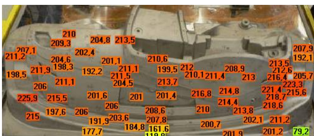
Fig. 1. Typical temperature field on the mould surface
