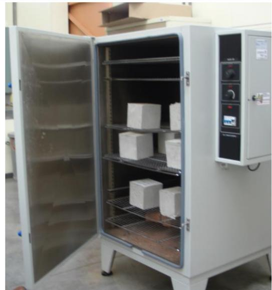
Fig. 3 Heating test setup in an industrial oven
