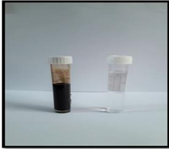
Figure (1): Image of CuO Nanoparticles Colloidal dissolved in PVP.
