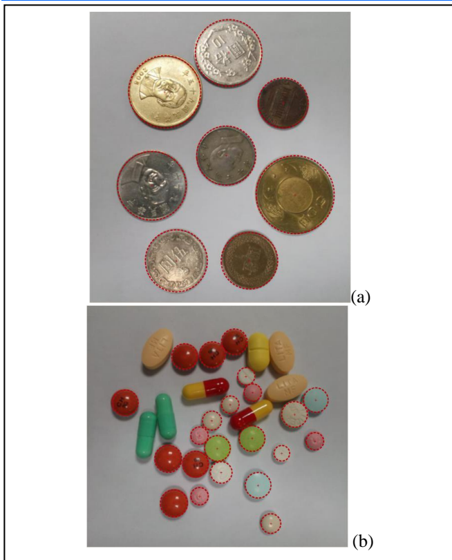
Fig. 12. Superimpose circles on the testing images: (a) coins, and (b) tablet drugs.
