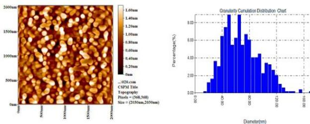
**Fig.( 2): 3D AFM image of and Granularity accumulation distribution chart of Ag nanoparticles ablation in ethanol.**
