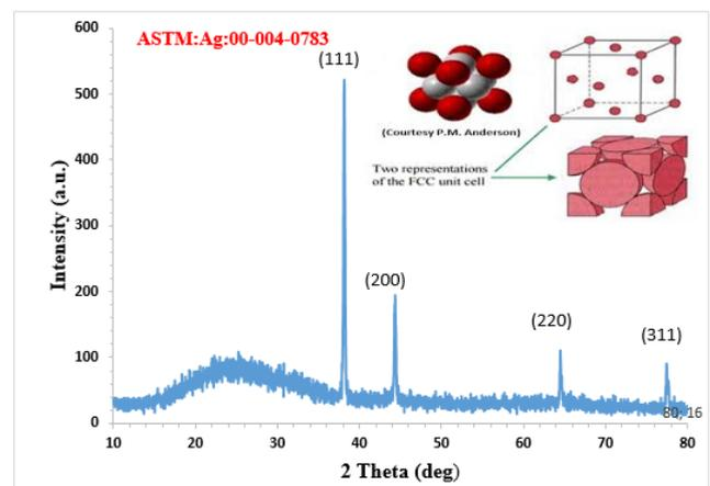
Figure (1) : XRD spectra of Ag thin film
