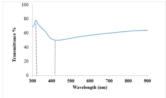
**Fig. (3): Optical transmittance for Ag thin film deposited on a glass substrate as a function of wavelength.**
