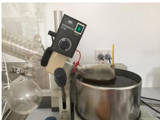
Figure 3. Solvent recovery using rotary evaporator
