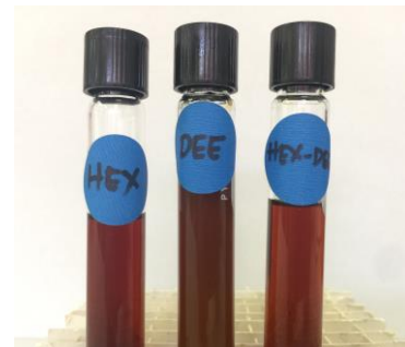
Figure 4. Emulsion phase observed in the FOG mixture extracted by DEE (middle tube)
