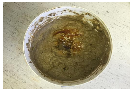
Figure 1. Dewatered grease trap waste
