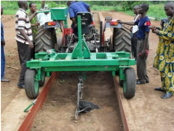
Fig. 2: Implement Carrier and Drive System during the Trial Test of the Instrumentation System
