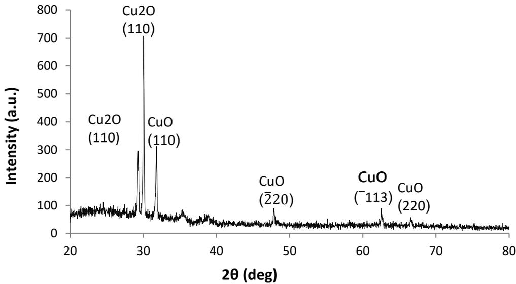
Fig. 4. XRD pattern for CuO thin film at 300°C
