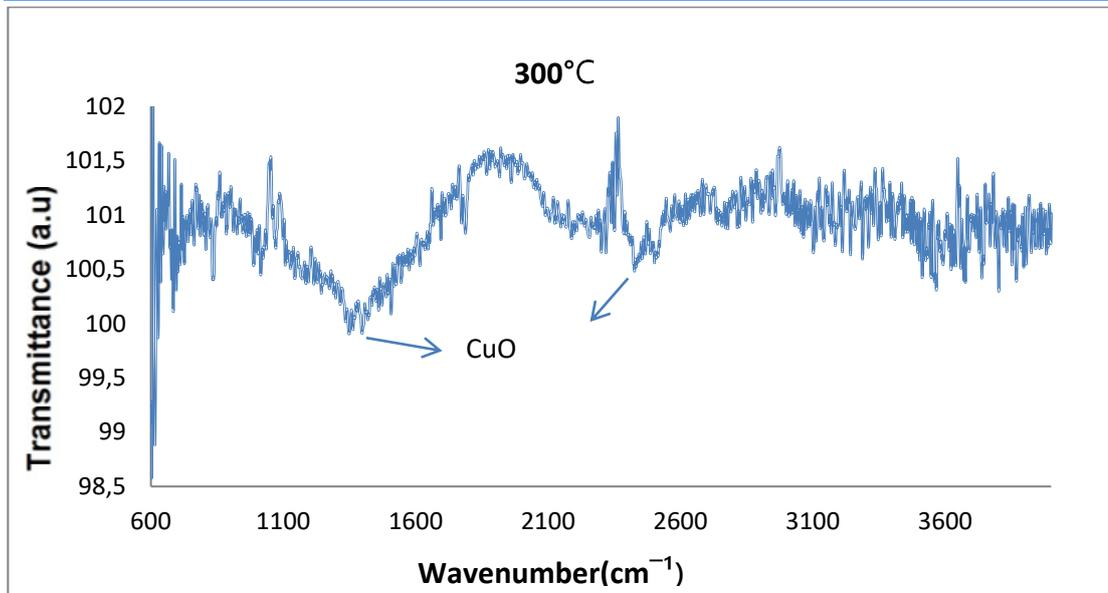
**Fig. 6: FTIR spectra of the CuO thin films at different annealing temperatures**
