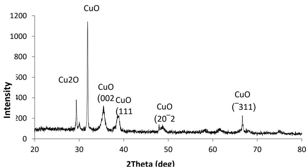
Fig. 1. XRD pattern of CuO thin film at as prepared
