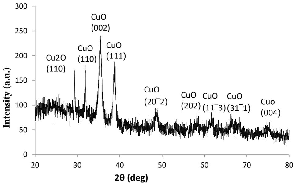
Fig. 2. XRD pattern of CuO thin film at 100°C
