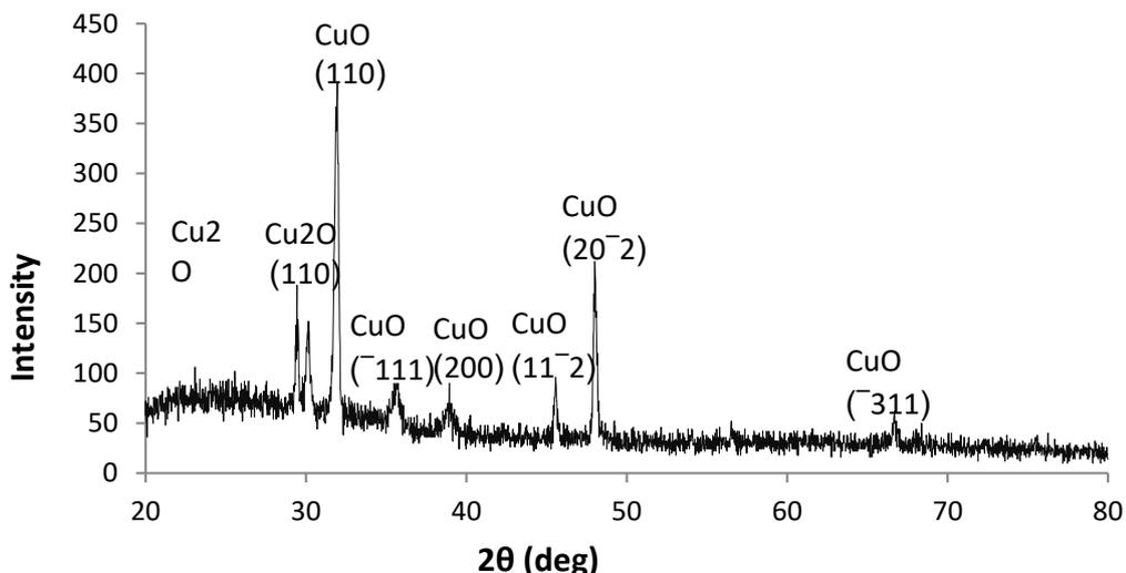
Fig. 3. XRD pattern of CuO thin film at 200°C
