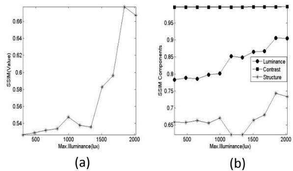
Figure (10) The Max. illuminance as a function of SSIM for the Value component in HSI color space (in a) and ( in b) the components of SSIM are (Luminance, Contrast and Structure),for first group images
