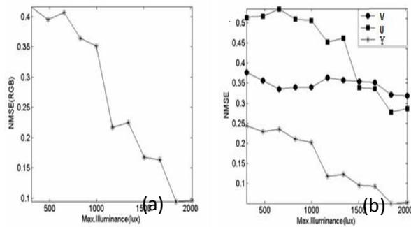
Figure (7) Relationship between Max.illuminance and NMSE (a) for RGB component and (b) for Y,U and V value components for first group images.
