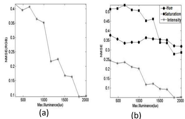
Figure (11) Relationship between Max. illuminance and NMSE (a) for RGB component and (b) for Hue ,saturation and intensity value components, for first group images.
