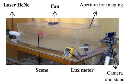
Figure (3) represents the system used to measure the amount of dust on the scene
