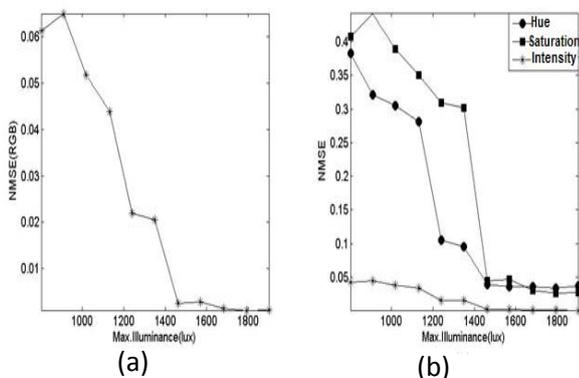
Figure (13) Relationship between Max.illuminance and NMSE (a) for RGB component and (b) for Hue,saturation and intensity value components, for second group images.
