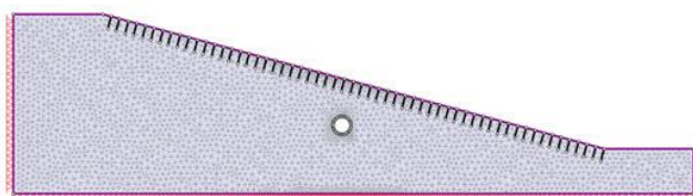
Fig. 1. The modeling of the circular tunnel with a diameter of 8 meter in the middle section of slope with dip of 15 degrees
