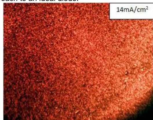
Fig. 5. Optical micrographs of porous silicon sample for 17min etching time, (M=1000X).
