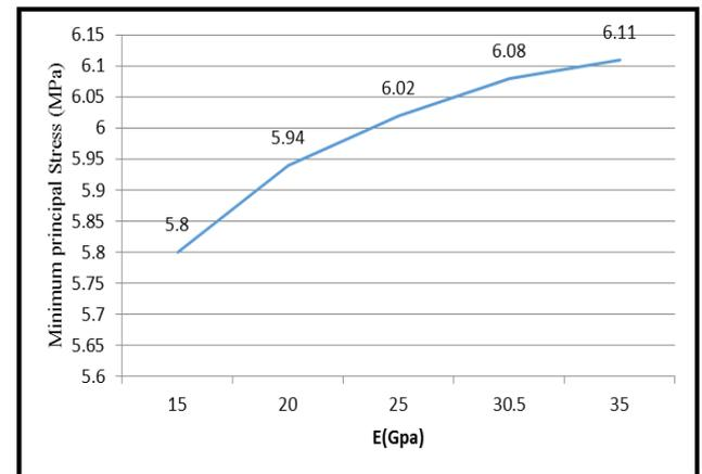
Fig. 19. Comparison of maximum principal compressive stress on the quay wall in five modes
