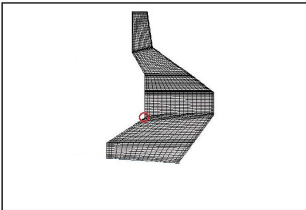
Fig.16. Location of maximum principal tensile stress on the body quay wall
