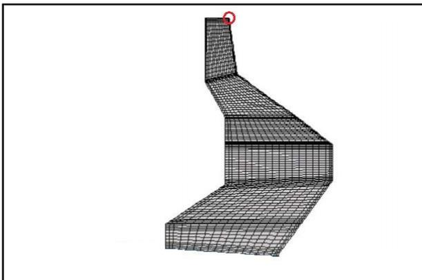
Fig. 17. Location of maximum horizontal displacement on the body quay wall
