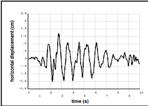
Fig. 9. Time history of quay wall maximum horizontal displacement with  $E=35$  Gpa
