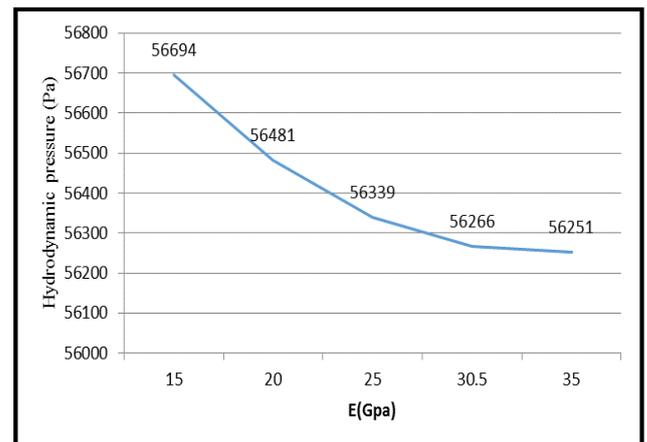
Fig. 20. Comparison of maximum hydrodynamic pressure exerted on fluid in front of the quay wall in five modes
