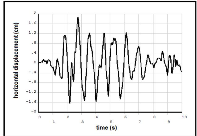
Fig. 6. Time history of quay wall maximum horizontal displacement with  $E=20$  Gpa
