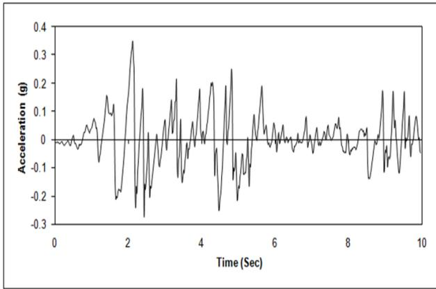
Fig. 3. North-south element of El centro earthquake
