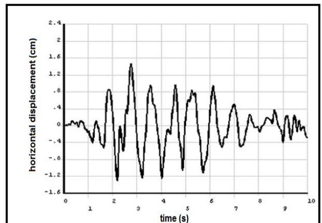
Fig. 8. Time history of quay wall maximum horizontal displacement with  $E=30.5$  Gpa
