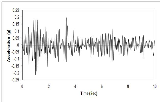
Fig. 4. Vertical element of El centro earthquake
