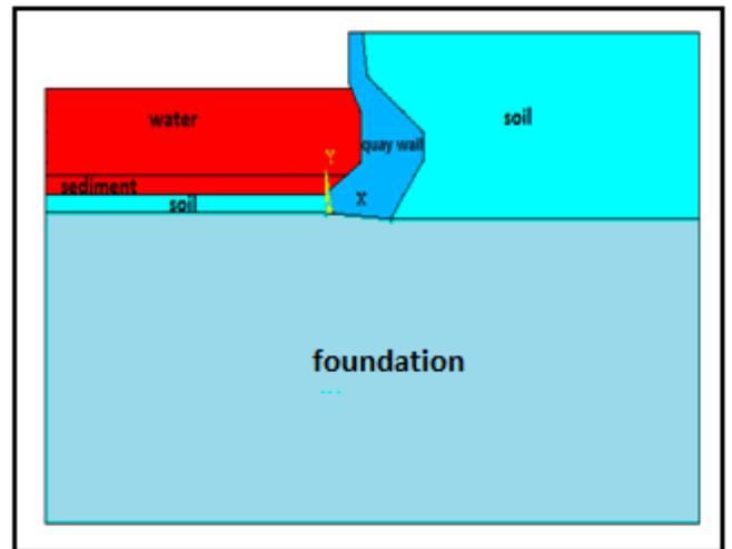
Fig. 2. Model geometry
