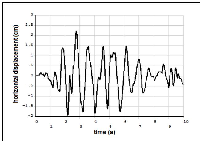
Fig. 5. Time history of quay wall maximum horizontal displacement with  $E=15$  Gpa
