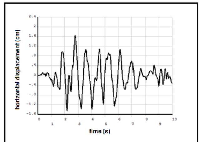
Fig. 7. Time history of quay wall maximum horizontal displacement with  $E=25$  Gpa
