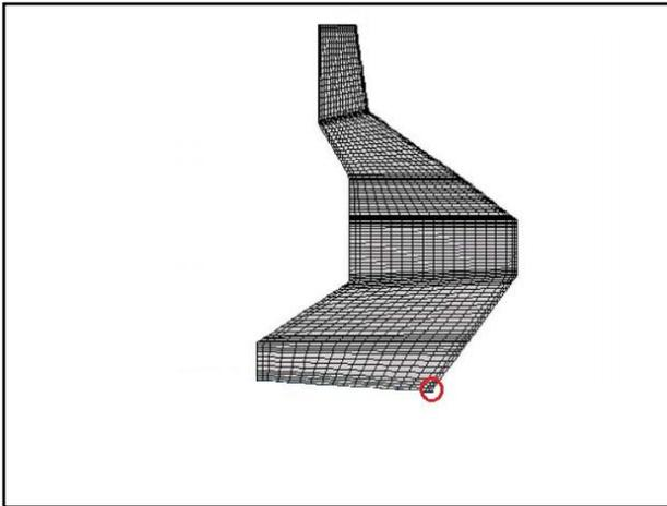
Fig. 15. Location of maximum principal compressive stress on the body quay wall
