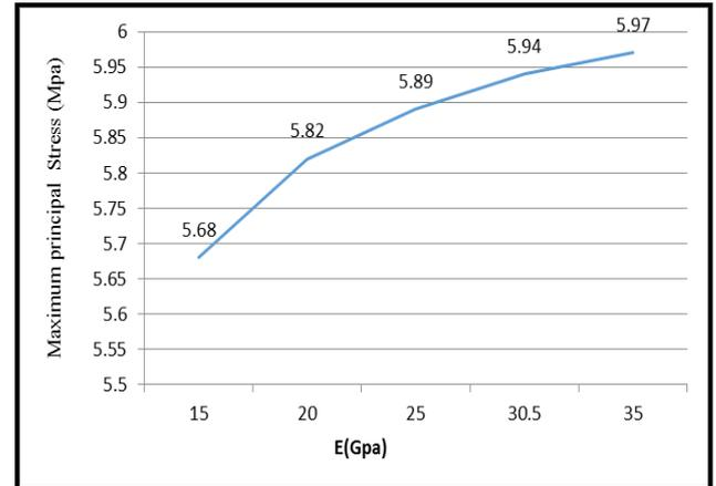
Fig. 18. Comparison of maximum principal tensile stress on the quay wall in five modes
