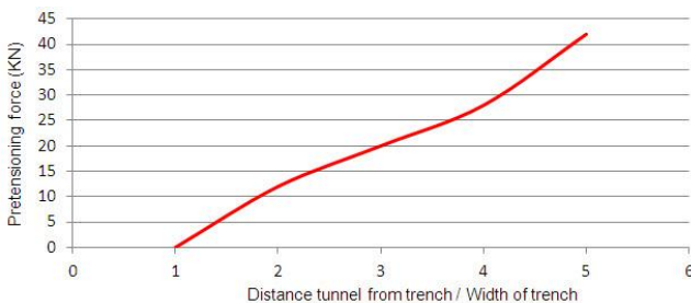
Fig. 9. The diagram shows the maximum of pretensioning force of anchors in terms of distance of tunnels from trench
