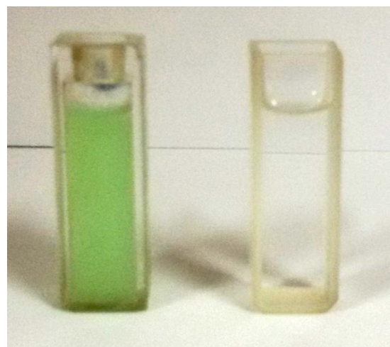
Fig.1: NiO freshly colloidal nanoparticles) which are prepared by chemical(left) which are prepared by chemical method and the solution(right)
