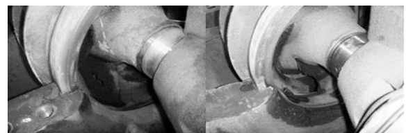
Fig. 3 Damage of impeller of split casing pump because of cavitation of recirculation
