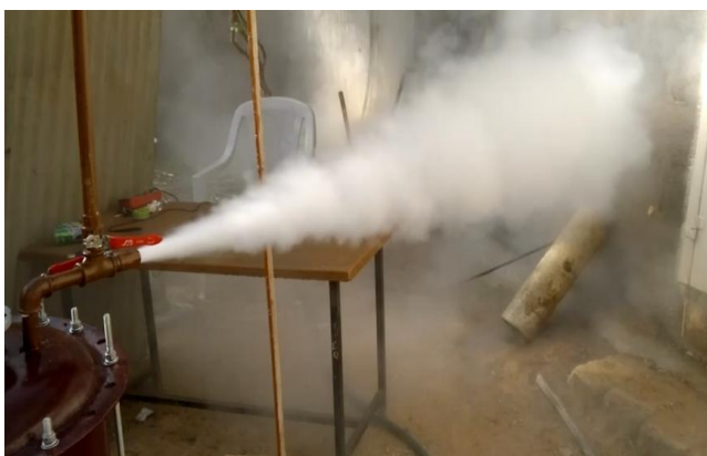
Fig. 10: Testing the boiler, steam power
