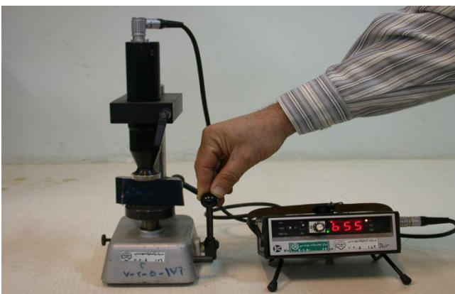
Fig. 3. The Krat-kramer hardness measuring during hardness measuring of the samples
