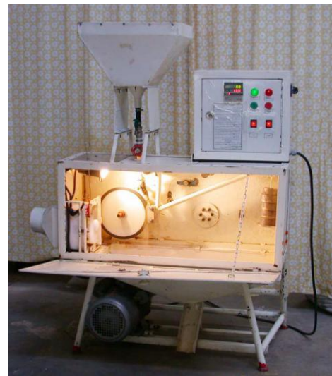
Fig. 1. Design and development a wear test of dry sand - rubber wheel
