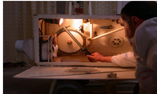
Fig. 2. Rubber Wheel diameter measured by a digital caliper
