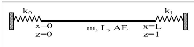
Fig. 2. Elastically supported beam
